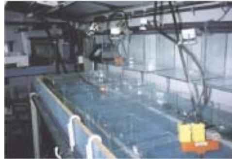
**Figure 3.5** Lincoln Creek side-stream fish bioassay test facilities nearing completion.
